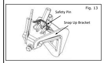
**NOTE: Secure Safety Pin to Snap Up Bracket**
